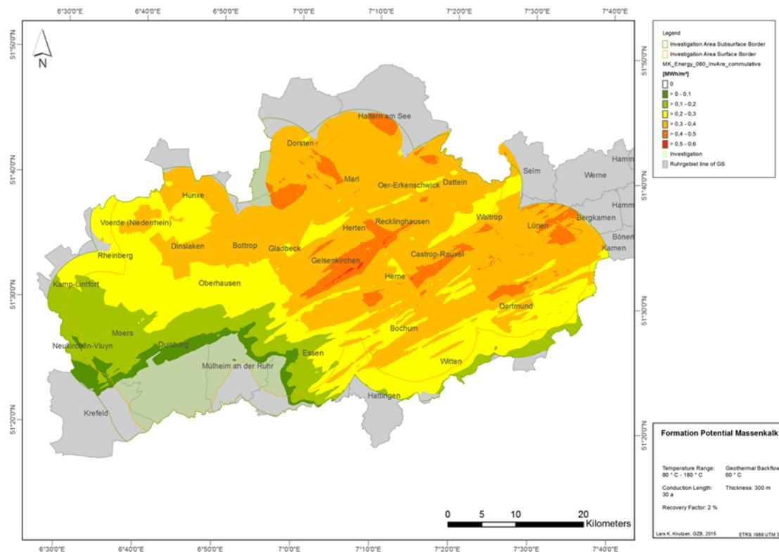
**Figure 8: Geothermal potential of Devonian limestone referred as *Massenkalk* with more than 300 m thickness, in 3,000 to 7,000 m depth, in temperature range of 80°-180°C (after Bracke et al., 2016)**
