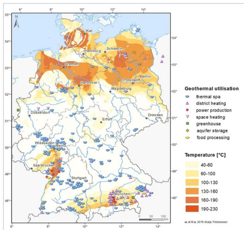
**Figure 6: Sites of deep geothermal utilization in Germany and neighboring countries. The background colors represent predicted temperature ranges of the respectively deepest identified geothermal resources in sedimentary or volcanic rocks (map generated in GeotIS, 2019).**
