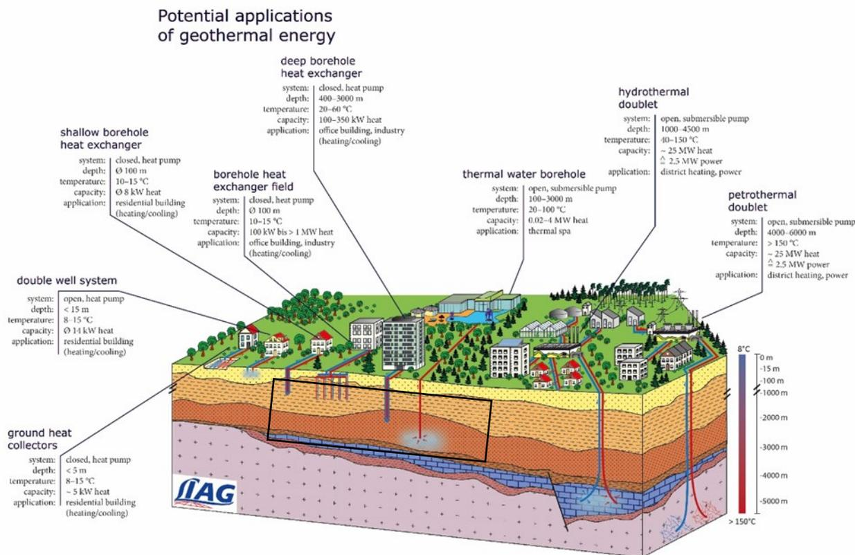
**Figure 10: Range of possible geothermal applications from shallow to deep resources in a play province with conduction dominated heat transport (adopted Weber & Moeck, 2019). Black box indicates mid-deep geothermal resources and its possible applications including well doublets, appropriate for small to medium scale heat provision.**
